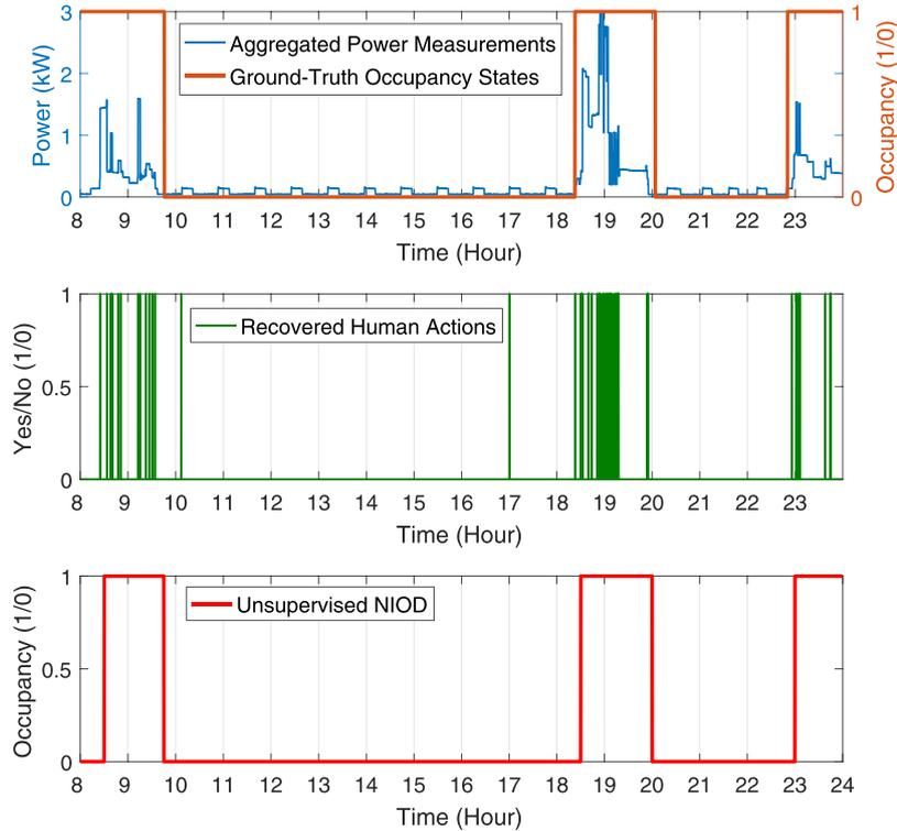
Fig. 5. Ground-truth occupancy states, recovered human actions, and estimated occupancy states from unsupervised NIOD. Note that the human actions recovered from false positive results have been filtered before being used for occupancy inference.
