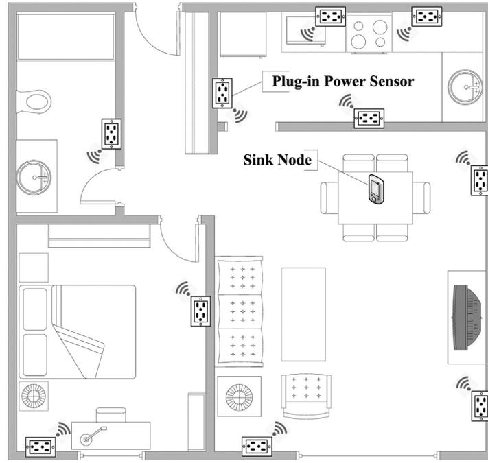
Fig. 3. Floor plan of an apartment and our smart home energy monitoring platform.
