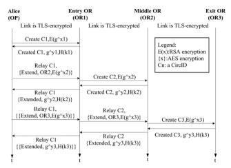
Fig. 3. Procedure of circuit construction.
