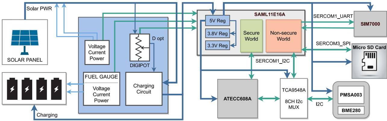
Fig. 5. Block diagram of the air quality monitoring device—STAIR.
