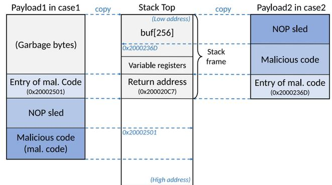
Fig. 2. Stack-based BOF attack for code injection.
