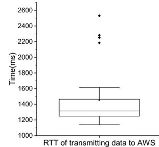
Fig. 11. RTT of transmitting data to AWS IoT through MQTTS protocol.
