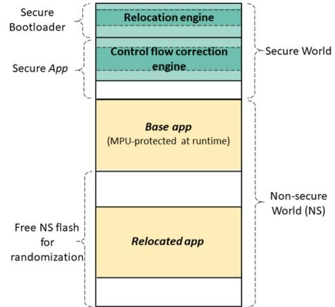
Fig. 8. Flash layout of an iASLR-enabled system.
