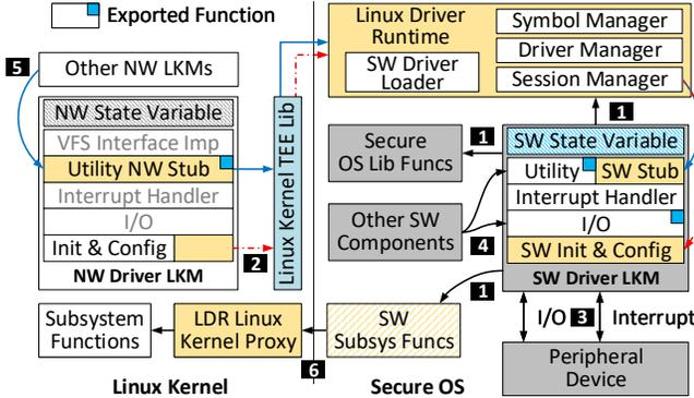
Fig. 4: **Workflow of SW Driver Execution.** White and grey to indicate NW and SW components respectively. Orange to indicate LDR newly-added parts. Blue to highlight state variable. Note that we exclude the security mechanisms to be discussed in §IV-E and §IV-F to illustrate a clear workflow.
