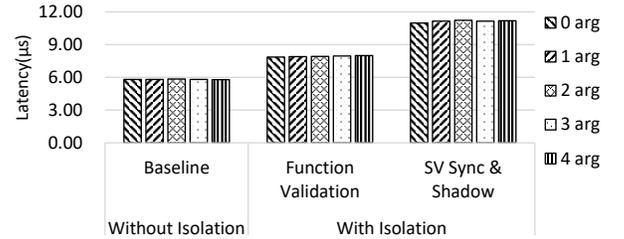
Fig. 13: Latency of Linux Function Redirection Mechanism
