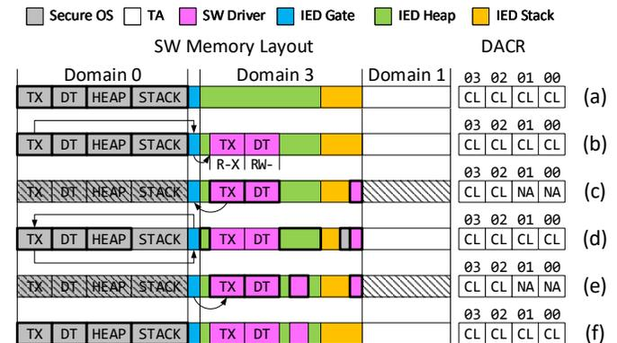
Fig. 11: Workflow of Calling `malloc()` from IED. Regions with thick boarder indicate regions that are currently activated and in control. TX stands for code. DT stands for data. IED gate is assigned to domain 2. IED is assigned to a new domain 3 and its memory layout consists of the IED heap and the dedicated stack.
